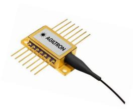
The 485nm series laser diodes are fabricated in a hermetically sealed 14-pin butterfly package. The laser diodes contain a thermoelectric cooler (TEC), and a thermistor to secure high-quality laser performance. The Laser Diodes Wavelength of 485±10nm, Output power: ≥20mW, Pigtail Type: 405-HP(Nufern) fiber with 900um loose tube, 1.0+/-0.1m, FC/APC connector. Our laser products are Telcordia GR-468 qualified and in compliance with RoHS Directives.
